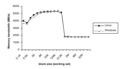
Figure 14: Extended copy transfer characterization (stride = 1)
