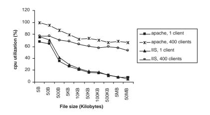
Figure 13: Web server CPU utilization
