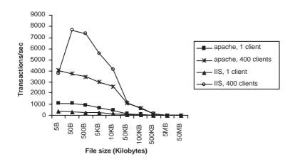
Figure 7: Web server transactions per seconds
