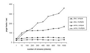
Figure 4: Page fault rate for 300kbps encoding rate
