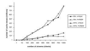
Figure 1: L1 cache misses for 56kbps encoding rate
