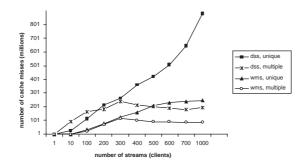
Figure 2: L1 cache misses for 300kbps encoding rate
